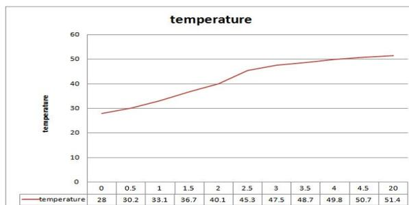
Figure 3. temp v/s time when peltier is heating
