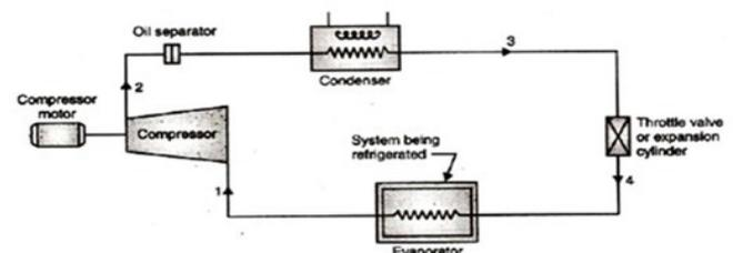
Figure 1. Schematic representation of VCR cycle
