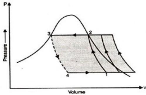
Figure 2. Pressure vs. Volume graph for VCR cycle
