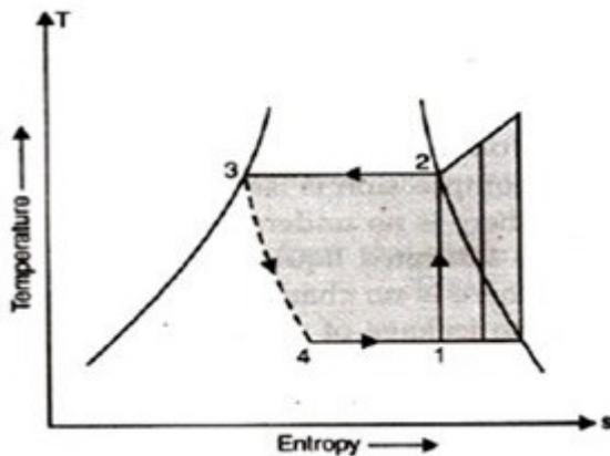
Figure 3. Temperature vs. Entropy graph for VCR cycle
