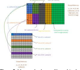
Figure 3. Memory load step of kernel in shared memory
