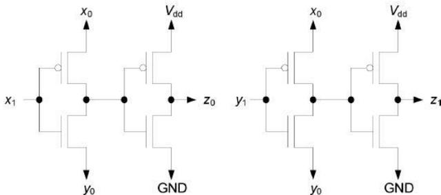
Figure.4: Two-pair two-rail checker
