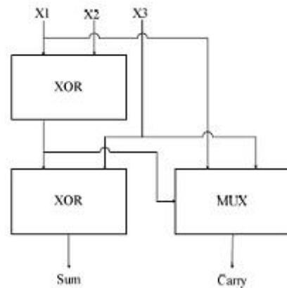
Figure 6: the internal architecture of 3-2 Compressor using XOR and Multiplexer
