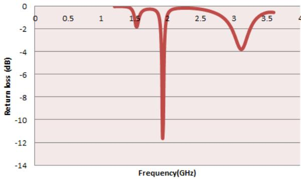
**Figure 3. Reflection Coefficient of the Proposed Antenna.**
