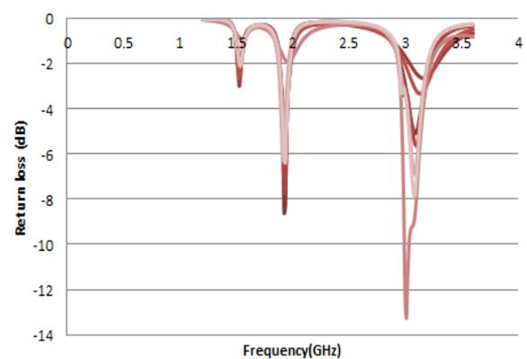
Figure 2. Parametric analysis of varying Coaxial feed positions-Reflection Coefficient of the Proposed Antenna.
