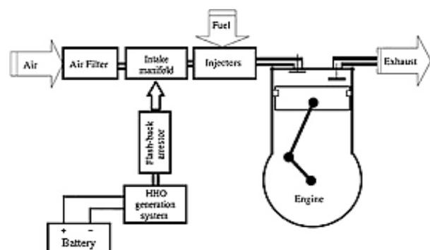
This works on the principal of electrolysis process. Electrolysis is the process that converts water to gas. The electrical supply for the process is used from your
