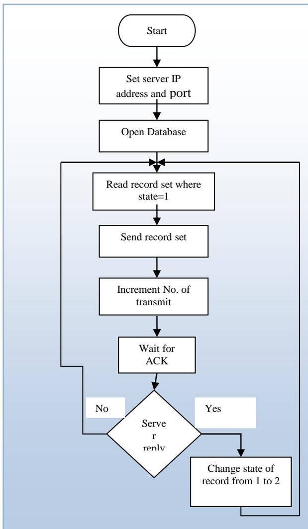
Figure 5: Flow chart of Transmitting Program (client)
