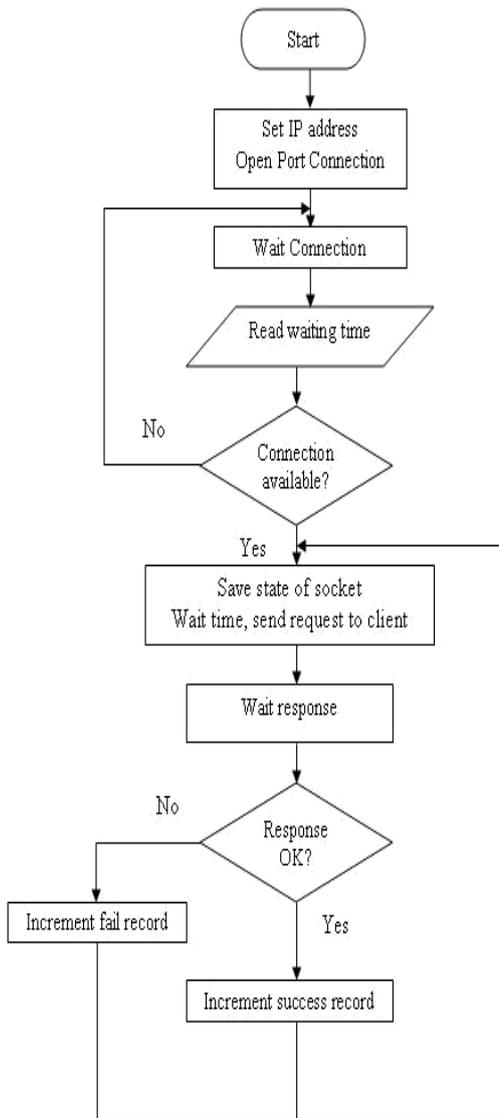
Figure 7 : Flow chart of Connectivity test program
