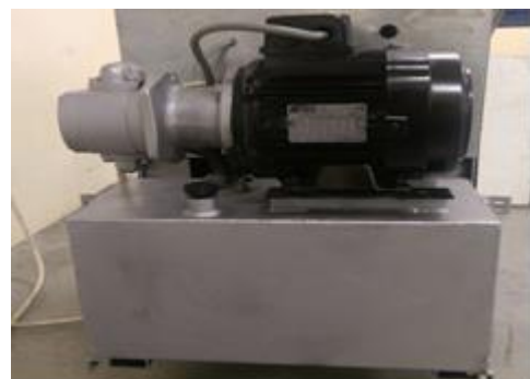
Figure 9: Hydraulic power pack
