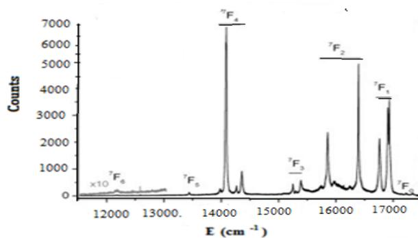
**Figure 4.** The fluorescence spectrum ( $5D_0 \rightarrow 7F_j$ ) of Eu<sup>3+</sup> in samples annealed at 830°C - the fluorescence spectrum of Eu<sup>3+</sup> in YAG
