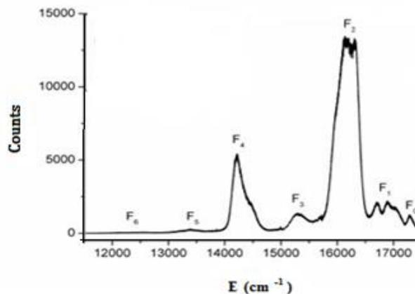
**Figure 3.** The fluorescence spectrum ( $5D_0 \rightarrow 7F_j$ ) of Eu<sup>3+</sup> in samples annealed at 800°C – amorphous state.
