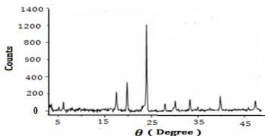
**Figure 2.** X-Ray Diffraction patterns of the sample heated at 1200°C.
