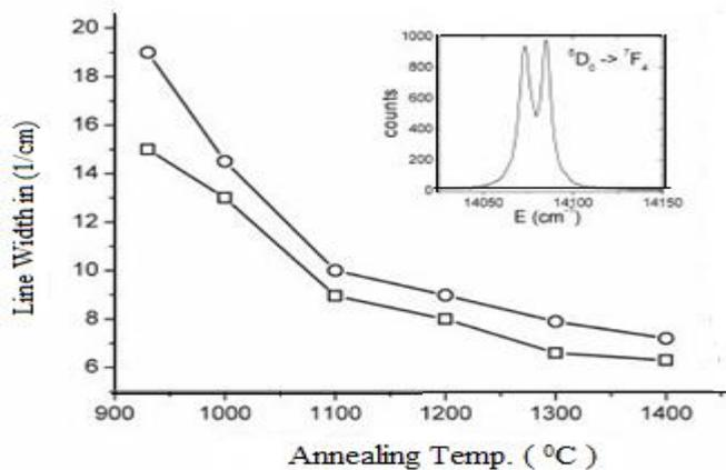
**Figure 5.** Dependence of line width with annealing temperature of two isolated fluorescence lines belonging to the transition  $5D_0 \rightarrow 7F_4$ . Inset: the two analyzed lines
