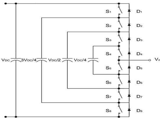
**Figure 2:** Flying Capacitor Multilevel Inverter (FcmlI)
