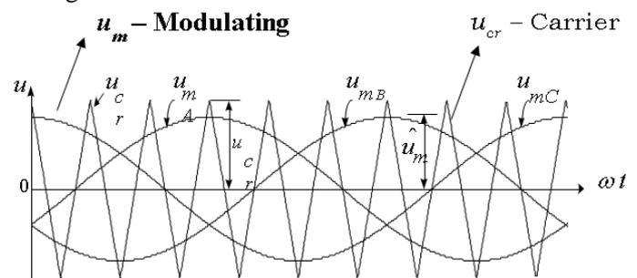
Figure 6: Modulating and Carrier Waves
