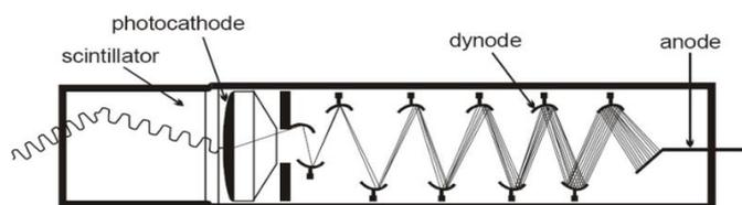
Fig.2 Scintillation Detector
