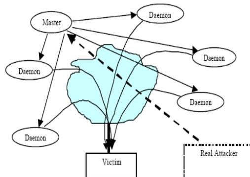
**Figure 1:** Distributed Denial of Service Attack Components
