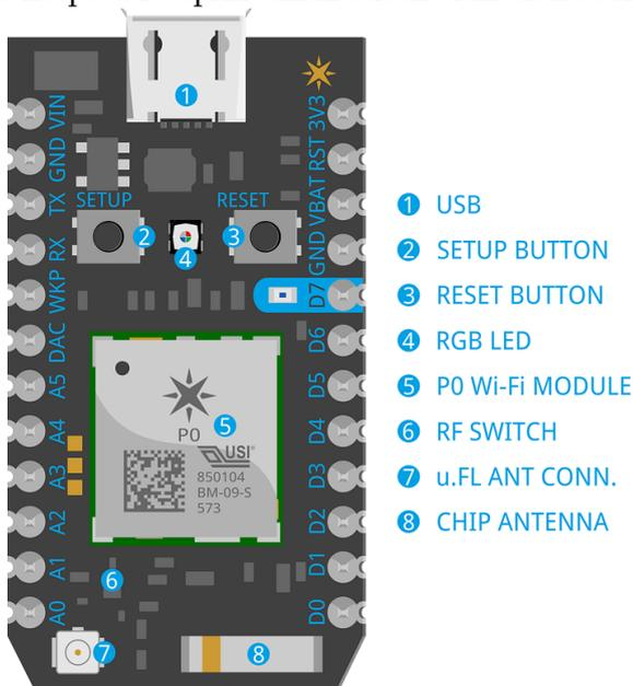
Figure: Particle Photon
