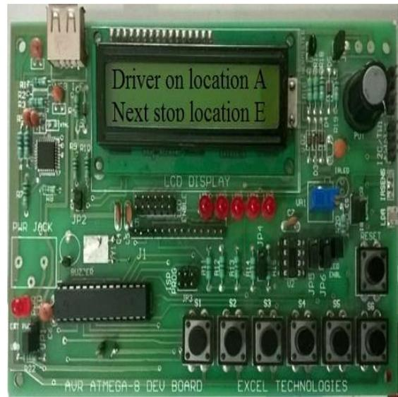
Figure 8: Hardware output on LCD display
