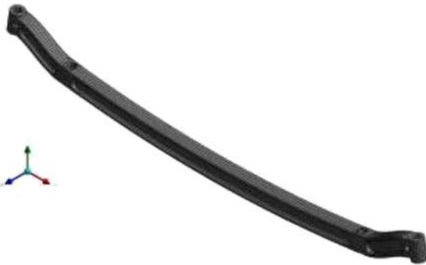
Figure 2. Finite element model of Front axle beam
