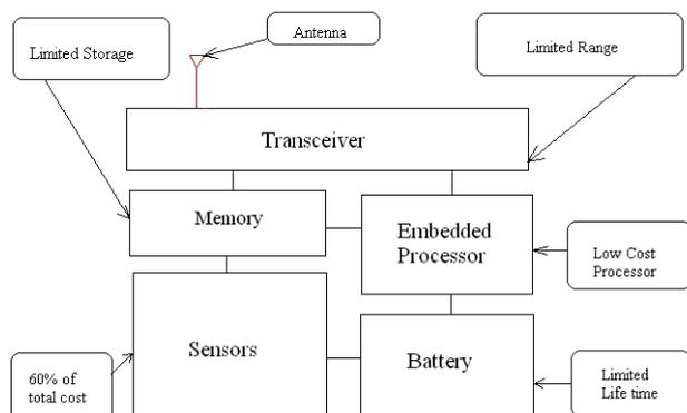
**Figure 1.** Components of a Wireless Sensor Node
