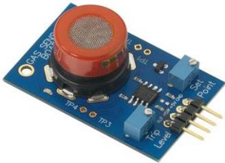
Figure 2. MQ7 gas sensor
