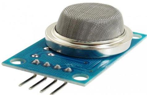
Figure 3. MQ6 gas sensor
