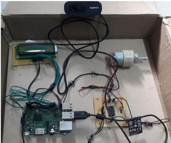
**Figure 20.** Road side speed sign monitoring and controlling project kit.
