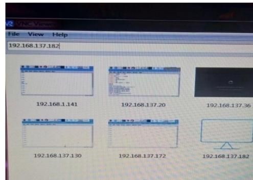
Figure 11. raspberry pi IP address from advanced IP scanner into vnc viewer.
