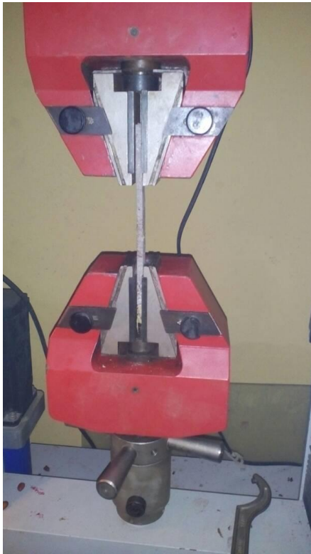
Figure 1. A composite board undergoing tensile testing
