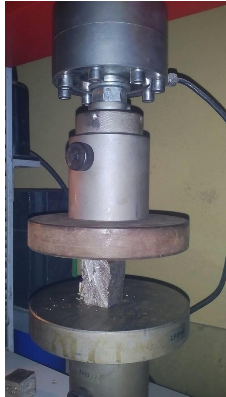
Figure 2. A composite board undergoing compression loading
