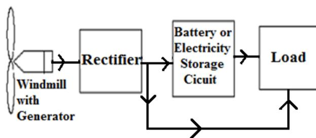
Figure 2: Block diagram of windmill electric power generation system
