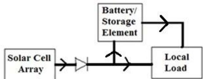
**Figure 1:** Basic solar (photovoltaic) electric power generation system
