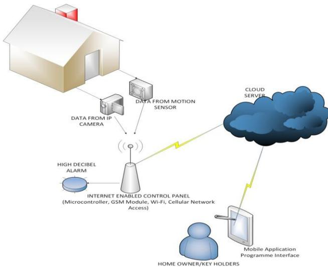
**Figure 2 :** The Proposed Analytics Enabled Anti-intruder System’s Model
