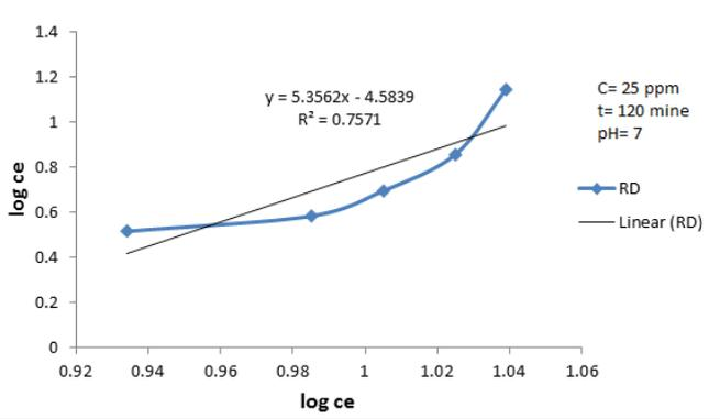
**Figure 8.** plot of Freundlich isotherm for RR removal from Water using bentonite clay.
