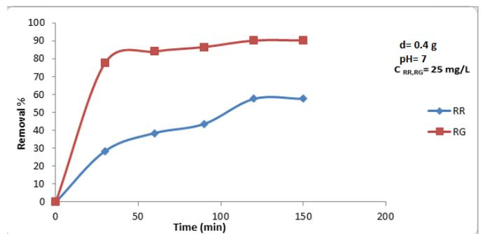
Figure 4. Contact Time Effect on the Removal efficiency of RR, RG
