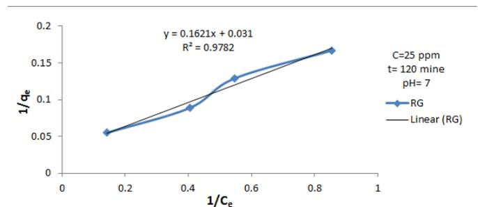
**Figure 7.** plot of Langmuir isotherm for RG removal from Water using bentonite clay.
