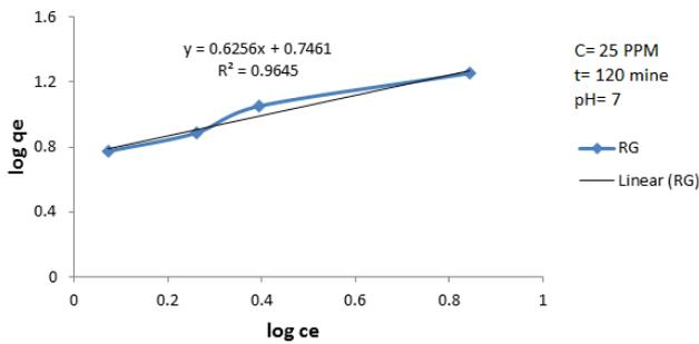
**Figure 9.** plot of Freundlich isotherm for RG removal from Water using bentonite clay.
