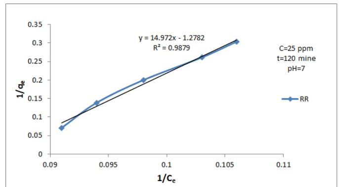
**Figure 6.** plot of Langmuir isotherm for RR removal from Water using bentonite clay.
