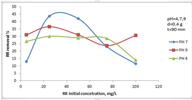
Figure 1. initial concentration effect on the removal efficiency of RR.
