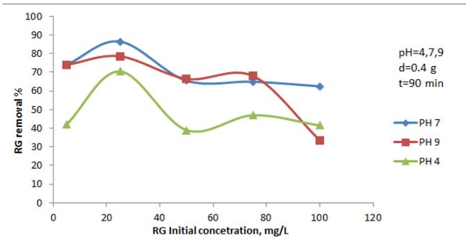
Figure 2. initial concentrations Effect on the removal efficiency of RG.
