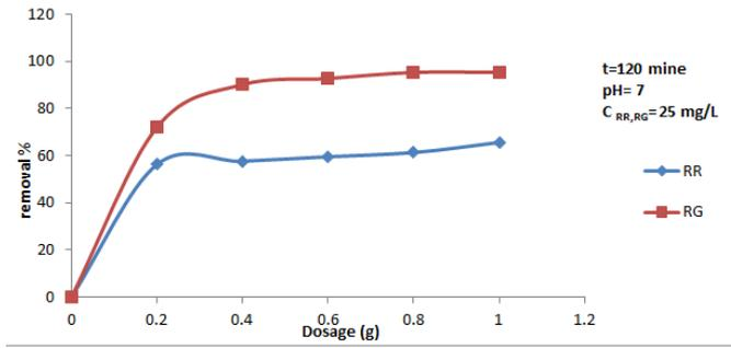
**Figure 5.** effect dosage the Removal efficiency of RR and RG.
