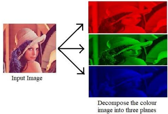
Figure 8. Decomposing of original image into R-G-B planes
