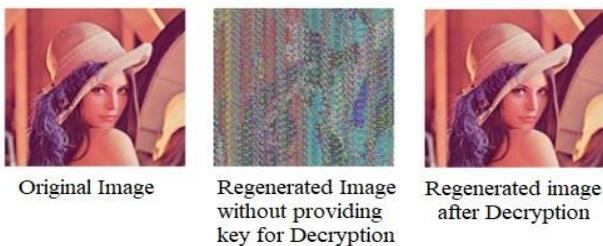
Figure 11. Effect of Decryption on the regenerated image
