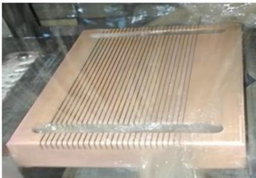
Figure 1. Mini channel copper block. Figure 2. Schematic diagram of mini channel refrigeration system.
