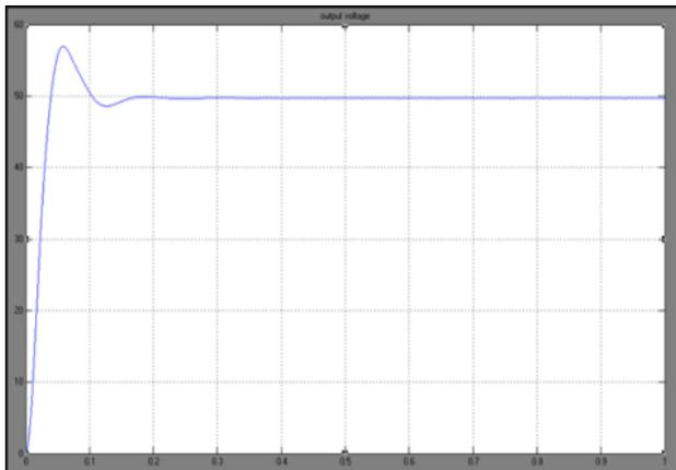
Figure 12. Output Voltage Waveform for the Proposed Converter
