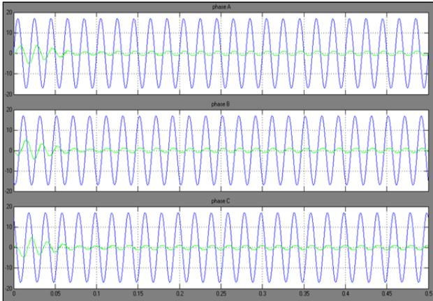
Figure 11. Input voltage and input current waveforms
