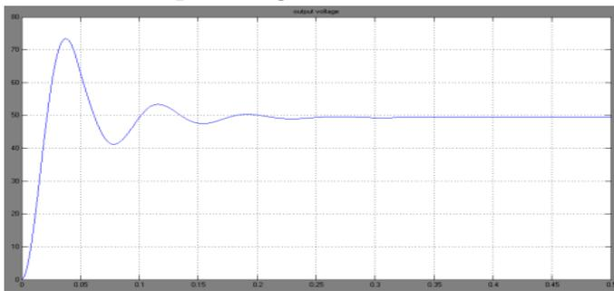
**Figure 6.** Output voltage waveform for open loop control
