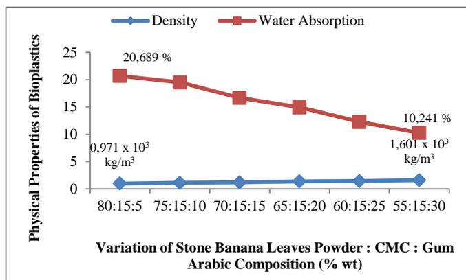
**Figure 1.** Test result physical properties (density and water absorption) of bioplastic based stone banana leaves powder/CMC/Gum Arabic on various variations composition
