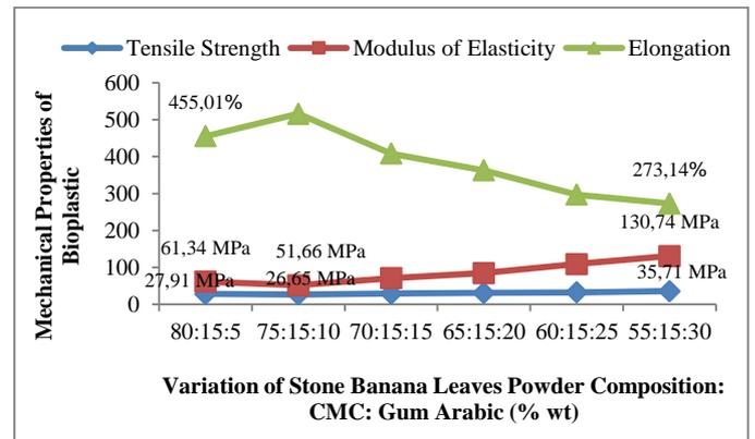
**Figure 3.** Test result mechanical properties (tensile strength, modulus of elasticity and elongation) of bioplastic based stone banana leaves powder/CMC/Gum Arabic on various variations composition
