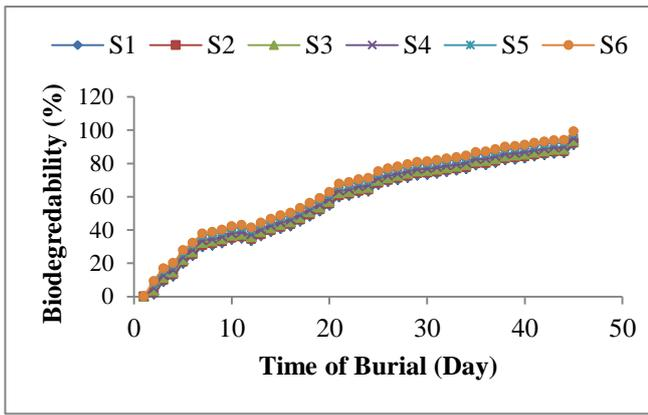
**Figure 2.** Test result biodegradability of bioplastic based on stone banana leaves powder/CMC/gum arabic on various variations of composition
