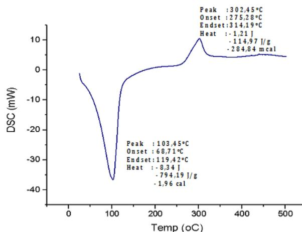
**Figure 4.** Thermal analysis (DSC) of bioplastic stone banana leaves powder/CMC/gum arabic on variation (55: 15: 30)%wt
