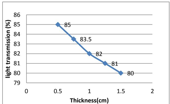
Figure 14: Graph of the relationship of transmission of light - vs - thick samples
