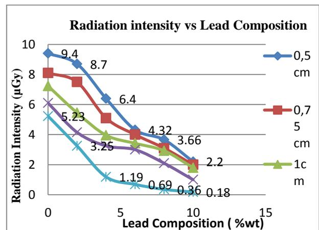
Figure 4: Relationship graph Radiation intensity - vs - Composition Sample voltage 40 kV
