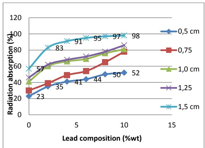
Figure 7: Graph of percentage of radiation absorption - vs - Sample composition of 40kV voltage
