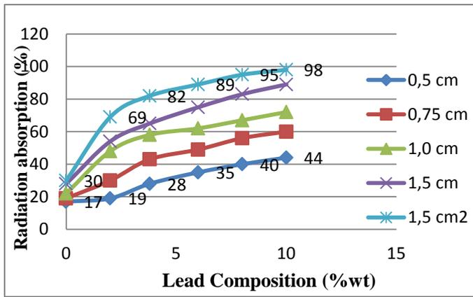
Figure 9: Graph of percentage of radiation absorption - vs. - Sample composition of 60kV voltage
