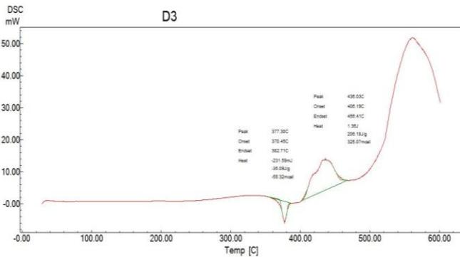
Figure 20: Graph of the results of DSC testing on composition samples (87: 10: 5)% wt lead.
