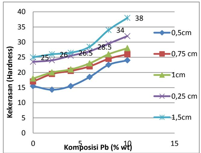
Figure 19 : Test graph of sample hardness - vs - Thickness of sample.
