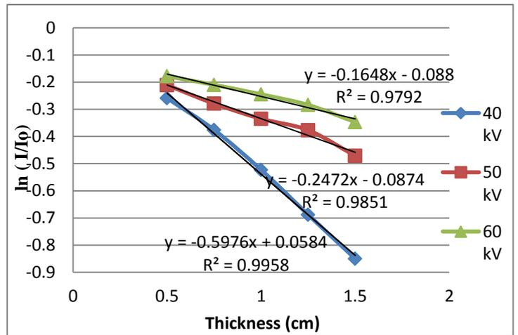
Figure 10: Graph of relationship of ln (I / Io) absorption of Radiation - vs - thickness of the sample
