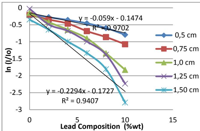
Figure 13: Graph of relationship of  $\ln(I / I_o)$  absorption of Radiation - vs - Composition of Samples at a voltage of 60 kV.
