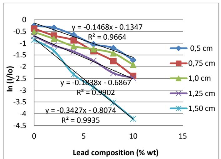
Figure 11: Graph of relationship of ln (I / Io) absorption of Radiation - vs - Composition of Samples at a voltage of 40 kV
