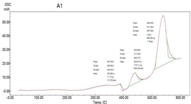
Figure 20: Graphs of DSC Testing on composition samples (95: 0: 5)% wt lead
