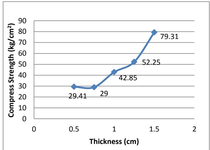
Figure 16: Graph of compressive strength - vs - thickness of the sample
