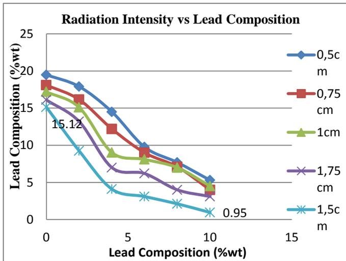
Figure 5: Correlationship graph Radiation intensity - vs - Composition Sample 50 kV voltage
