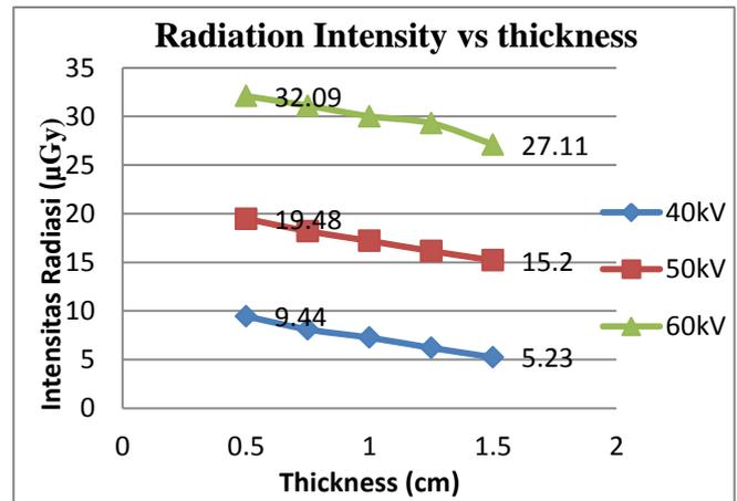
Figure 3: Radiation intensity - vs - Thickness of the sample
