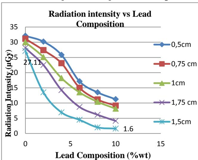
Figure 6: Relationship graph Radiation intensity - vs - Composition Sample voltage 60 kV
