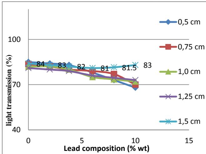
Figure 15: Graph of the relationship of light transmission - vs - sample composition
