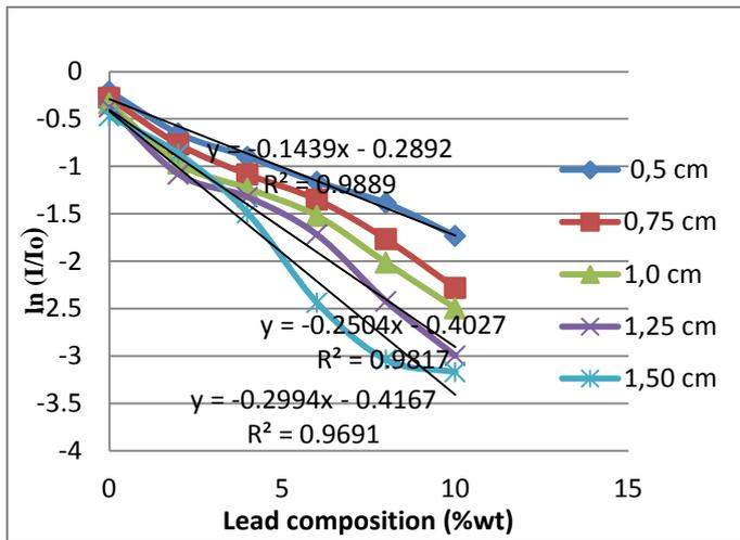
Figure 12: Graph of relationship of  $\ln(I / I_o)$  absorption of Radiation - vs - Composition of Samples at a voltage of 50 kV
