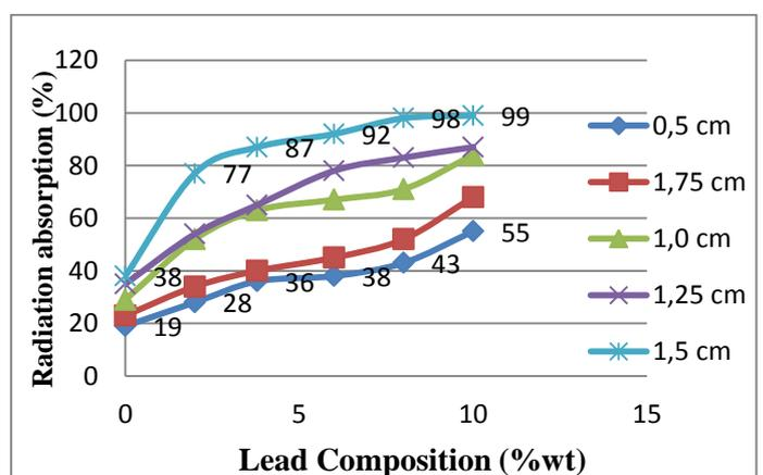
Figure 8: Graph of percentage of radiation absorption - vs - Sample composition of 50kV voltage
