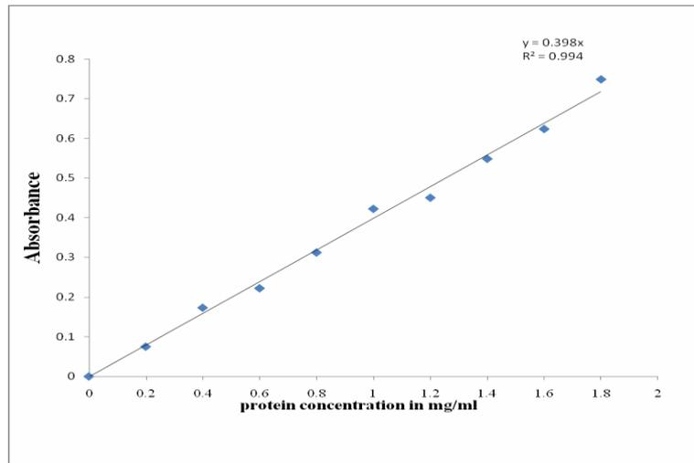
**Figure 3.** Protein Standard Curve, Using 2 mg/mL Bovine Serum Albumin (BSA)
