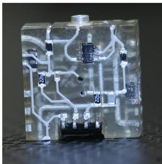
**Figure 1:** 3D Printed Signal Conditioning Circuit
