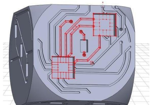
**Figure 3:** Electronic Circuit Mechanically Designed into Substrate.
