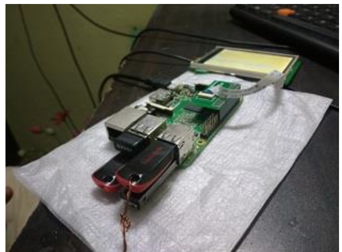
Fig 7: Raspberry Pi board connected to three Pendrives
