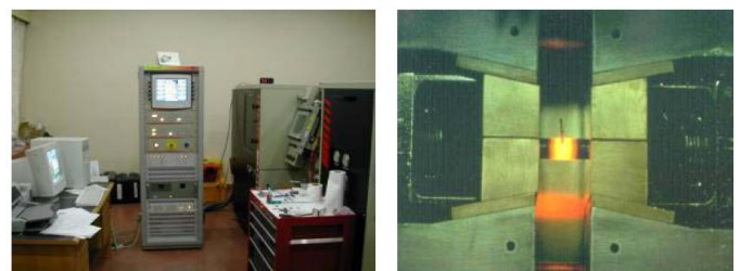
Figure 3: Thermo mechanical simulator (Gleeble-3500) for isothermal forging of the samples
