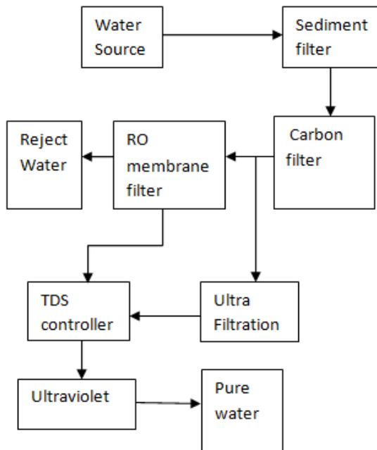
**Figure 1.** Schematic diagram of the stages in Reverse Osmosis
