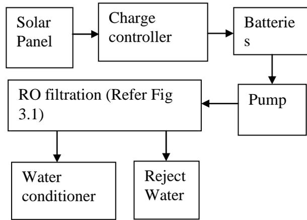
**Figure 5.2.2. Schematic representation of proposed Reverse Osmosis filtration and water conditioner**
