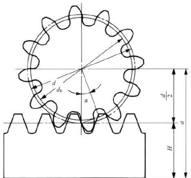
**Figure 2.2. Rack and pinion**
