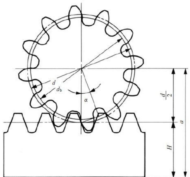
Figure 2.2. Rack and pinion
