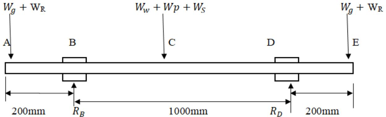
Figure 2.3. The bending moment on the shaft
