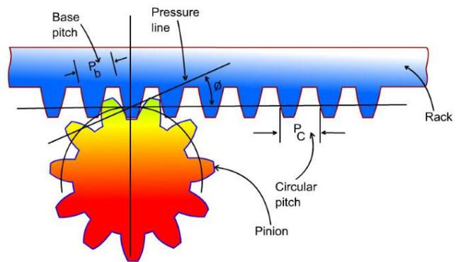
**Figure 2.1. Rack and pinion**
