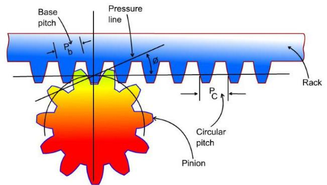
Figure 2.1. Rack and pinion
