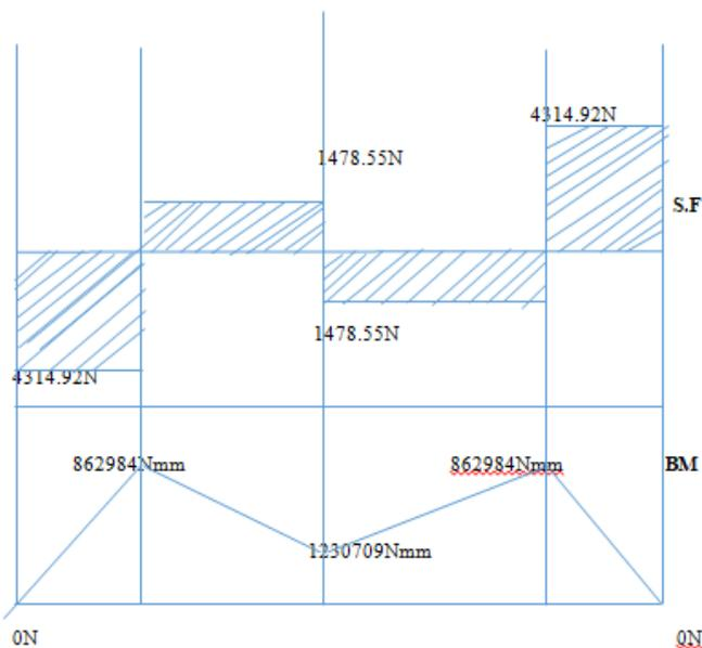
Figure 2.4. Shear Force And Bending Moment Diagram Of The Shaft.
