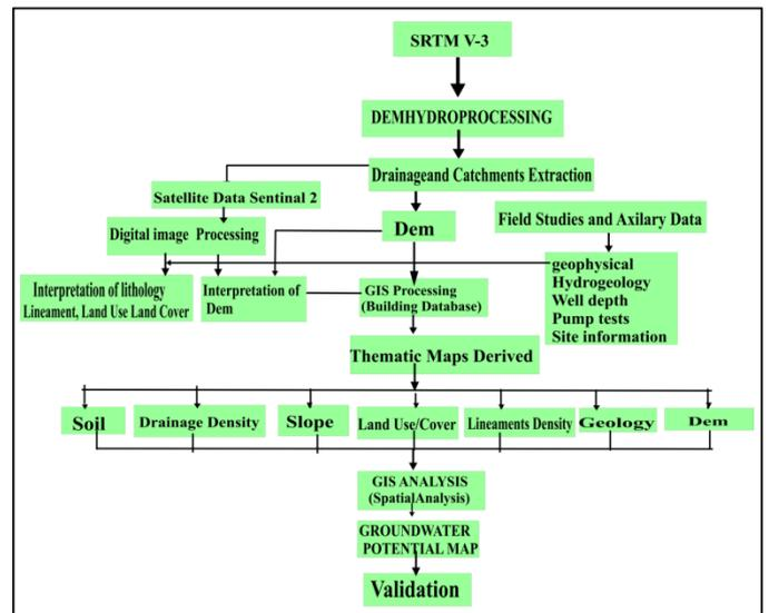
Figure (4) : Flow Chart Showing Data and Methods Employed for the Study
