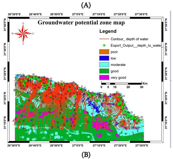
Figure (13). Validation of Groundwater Potential Zones Map by Depth to Water (B) and Well (A)
