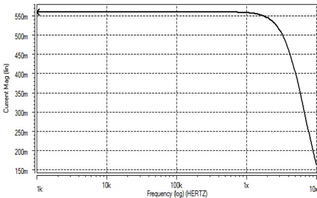
Figure. 5. Frequency response of  $I_{out} / I_{in1}$
