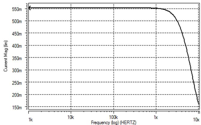
Figure. 6. Frequency response of  $I_{out} / I_{in2}$
