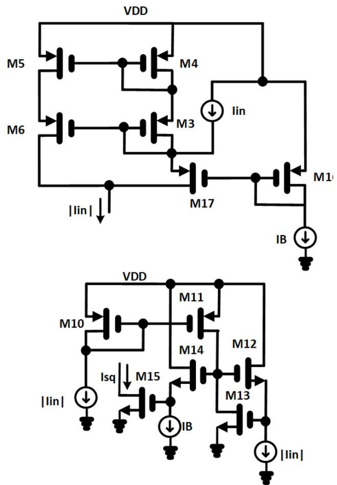
Figure. 3. The squarer with the absolute-value circuit
