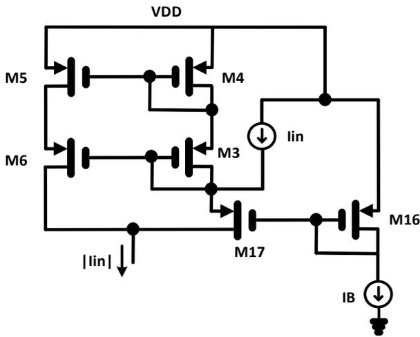
Figure. 2. Absolute-value circuit of the RMS-to-DC converter.
