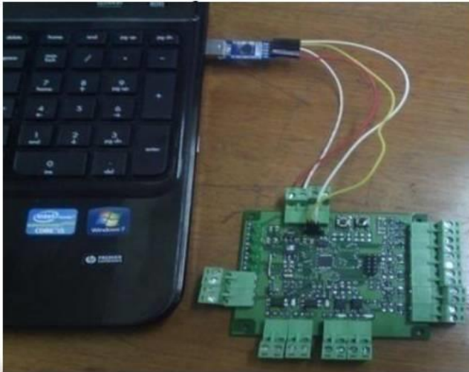
Figure 7. Integrated Unit of designed Temperature Scanner
