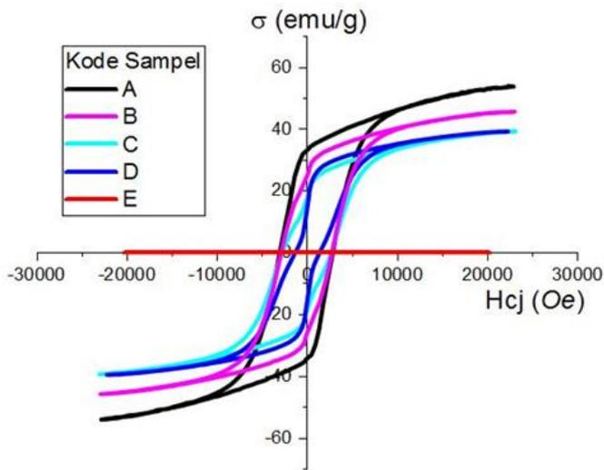
Figure 4. The magnetic field hysteresis curve (Ms), (Mr), (Hcj) influences the addition of % ZnO to BaFe<sub>12</sub>O<sub>19</sub>.
