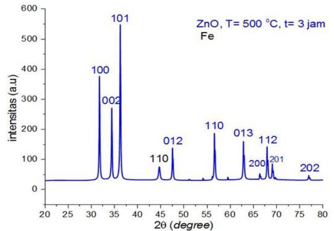
Figure 2. XRD pattern of ZnO (filler)
