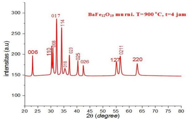
Figure 1. XRD pattern of BaFe<sub>12</sub>O<sub>19</sub> (matrix)
