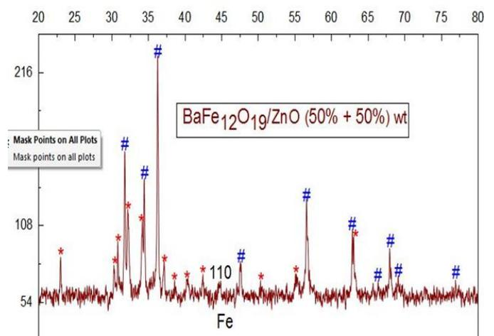
Figure 3. XRD pattern of BaFe<sub>12</sub>O<sub>19</sub>/ ZnO composite
