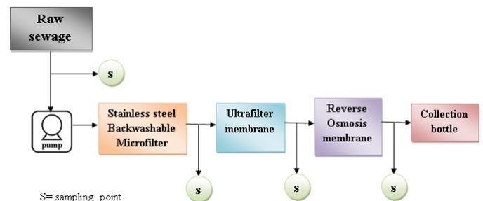
Figure 1: Experimental Setup
