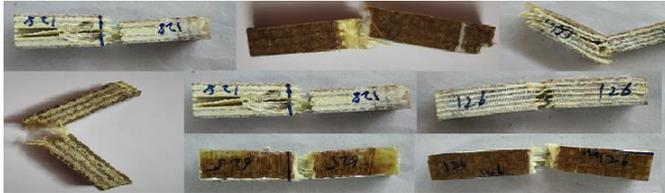
Figure 4. test specimens after izod and charpy impact tests
