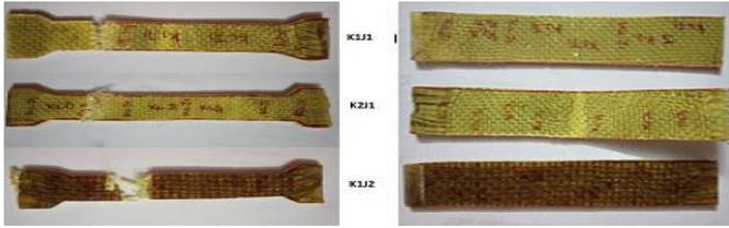
Figure 3. test specimens after tensile and flexural tests
