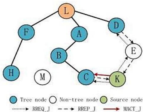
Figure 3 : Link Repair Mechanism of MAODV
