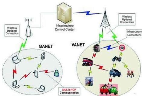
Figure 1 : Architecture of MANET and VANET.
