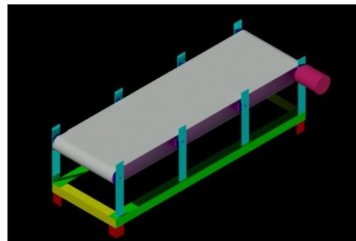
**Figure 9.** Conveyer belt with motor attached.
