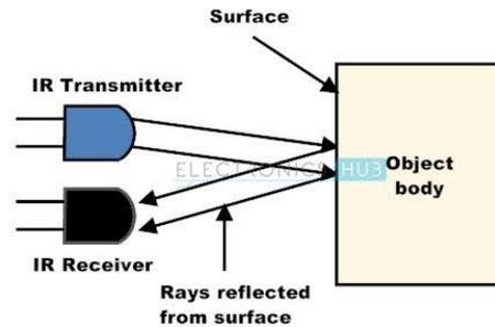
Figure 3. Working of IR Sensors.
