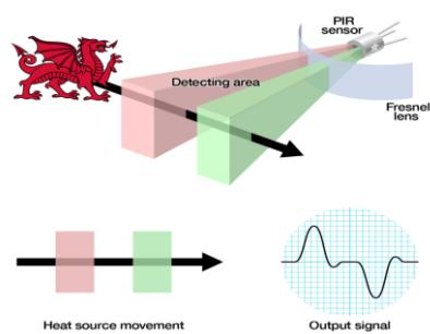
**Figure 4.** Working of PIR Sensor
