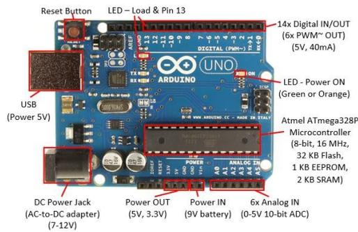
**Figure 8.** Arduino Board.
