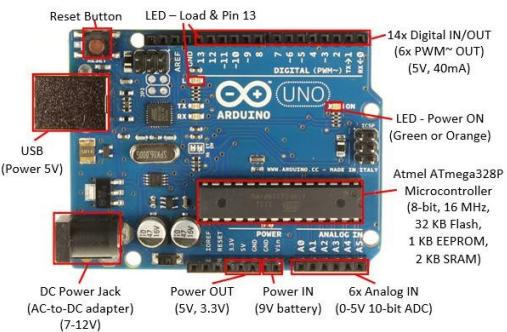
**Figure 8.** Arduino Board.
