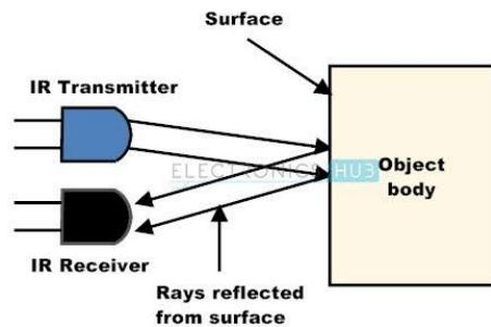
**Figure 3.** Working of IR Sensors.
