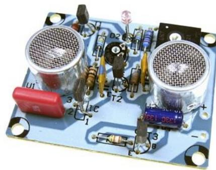
**Figure 7.** Ultrasonic Sensor
