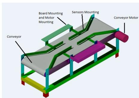
**Figure10.** Conveyor Belt with separation tray.
