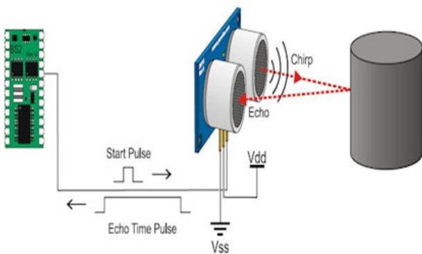
**Figure 6.** Working of Ultrasonic Sensor.
