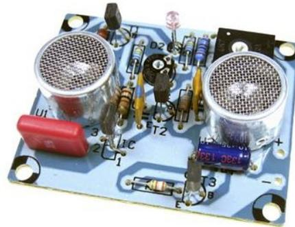
Figure 7. Ultrasonic Sensor
