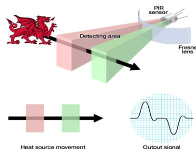
Figure 4. Working of PIR Sensor
