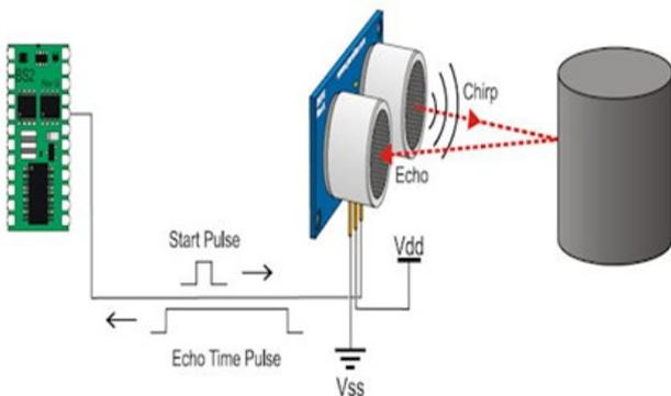
Figure 6. Working of Ultrasonic Sensor.
