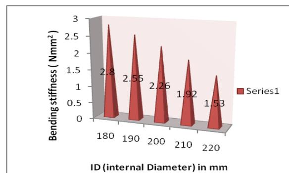
Figure 1: Effect of internal diameter on bending stiffness
