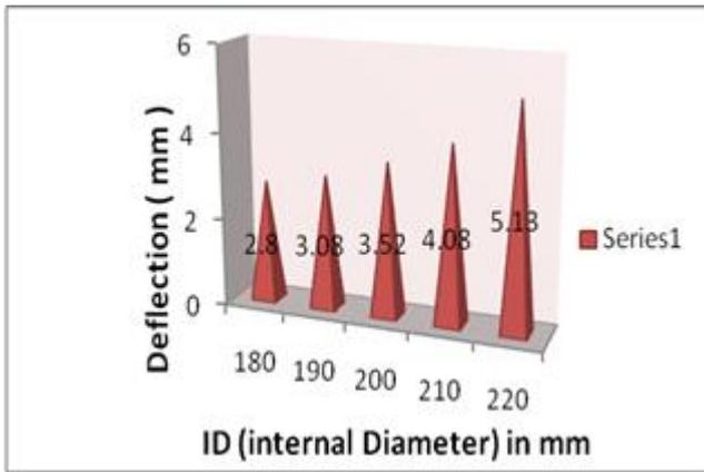
Figure 2 : Effect of internal diameter on deflection
