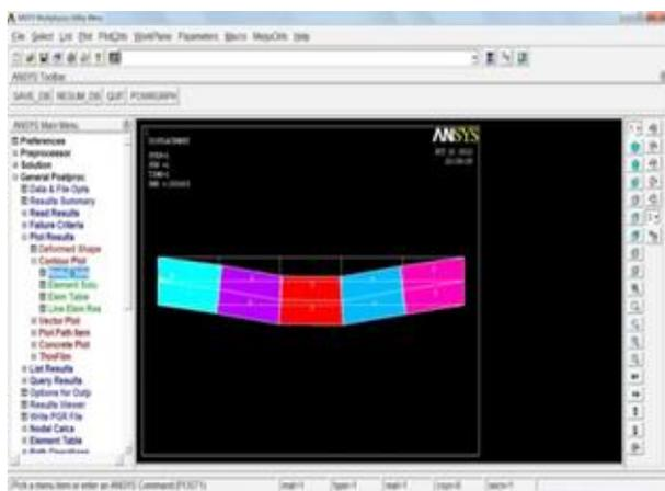
Figure 3 : Simulation results :Shaft bending with ID 230mm
