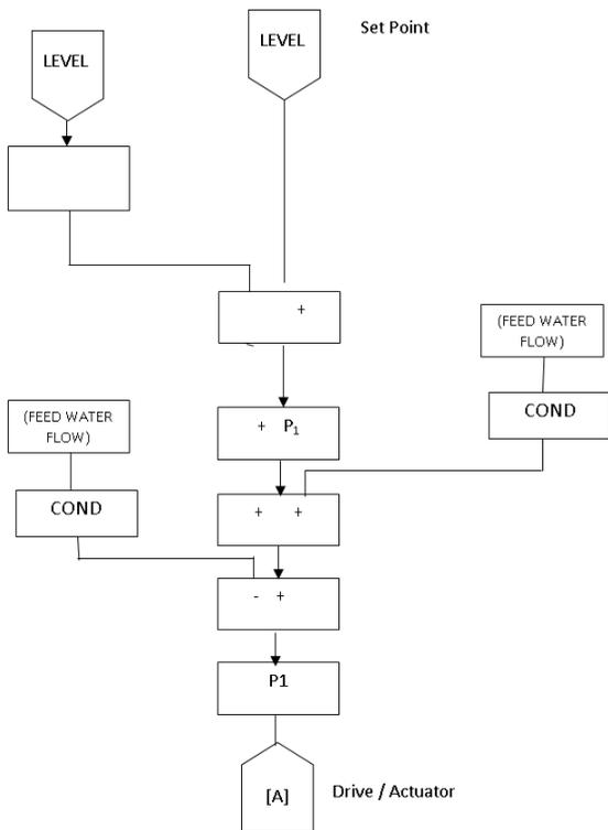
**Figure 1:** Shows the Drum Level Three Element Controller
