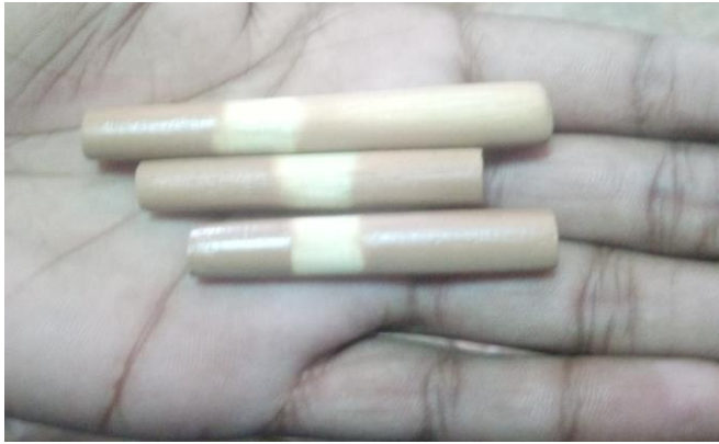
Figure 3. Wooden masking plug
