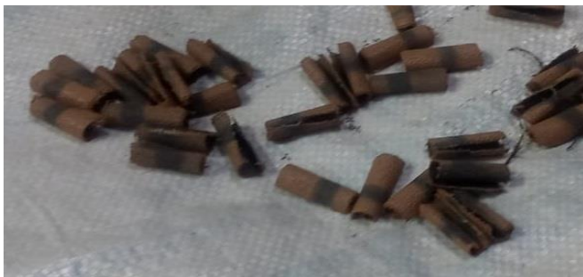
Figure 2. Paper masking plug
