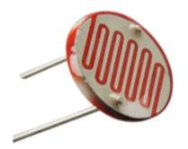
Fig.4: Light Dependent Resistor (LDR)
