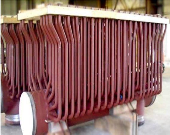
The modification of front wall tubes headers that the addition of tubes to increase the area so that the increasing in the boiler efficiency. The Increases the area to increasing the boilers efficiency. E.g. the old tube size is 76.2OD\*4.06\*12525 and new tubes size is 76.2OD\*4.06\*13129.when the area increasing to increase the boilers efficiency. The heating area increasing this condition to increasing efficiency by 2.08%
