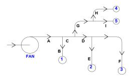
Figure 1. Typical air conditioning duct lay-out
