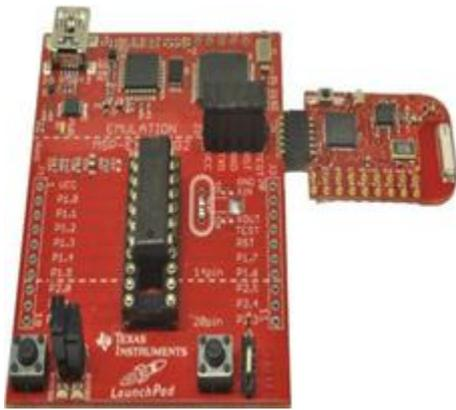
**Figure 6 :** MSP-EXP430G2 LaunchPad with Attached eZ430-RF2500 Target Board
