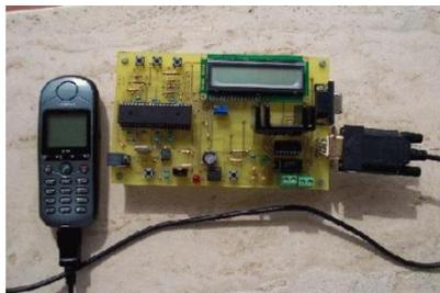
**Figure 4 :** Interface Module of GSM Kit
