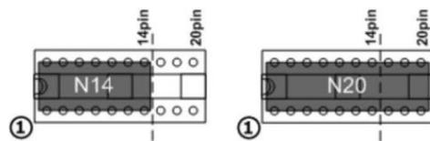
**Figure 5 :** Insert Devices into Target Socket
