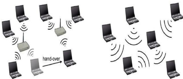
(a) An infrastructure network with two base stations. (b) A mobile ad-hoc network. Fig 1 Infrastructure and ad-hoc networks
