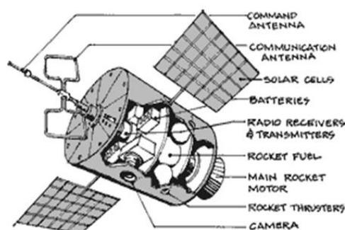
Messages sent to the satellite from a ground station are "uplinked"; messages transmitted from the satellite to Earth are "downlinked."
