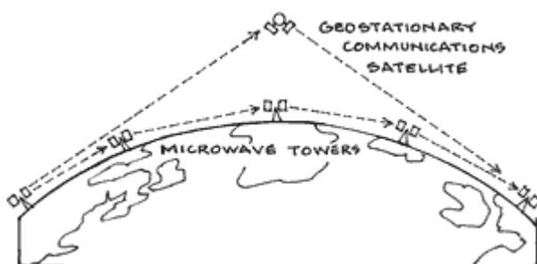
dissipate into the ocean. Over short distances, we erect microwave towers every 25 miles or so to act as "repeaters" to repeat and boost the signal. Think of a geostationary communications satellite as a repeater in the sky.
